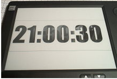
Figure 4: An E-ink Showing the Ghost of a Previous Image (Source: Wikipedia, 2010).
